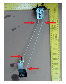
A. Carefully straighten out the four bends as shown. The reshaped unit should be slightly off vertical. Be careful not to damage electrical wire attached to low level arm.
