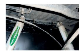
21. Raise and support rear of fuel tank so that mounting points are pushed against corner gussets of chassis. Centralise fuel tank and drill holes through chassis on each side using mounting holes in fuel tank as a guide.
