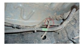
14. Using a hammer, bend seam backwards about 5mm to allow clearance for tank.
