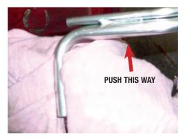
F. Carefully support pipes in vice as shown and bend pick up assembly in direction shown in photograph to allow pipes to sit closer to top of fuel tank once installed.
