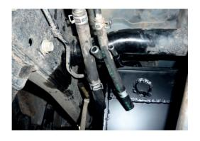
24. Cut fuel filler and fast fill breather hoses to required length and refit.
