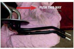
17. Install fuel sending into new tank making sure the float clears the bottom of the tank.
