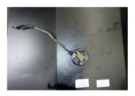
18. Refit filter to fuel pick up and install assembly to fuel tank making sure the pick up is close to but not touching the bottom of the fuel tank.
