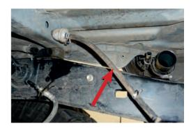
10. Remove fuel tank support strap brackets.
