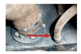
6. Unclip and disconnect fuel sender wires.
