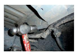
15. Bend pick up and return lines under cross member as shown.
