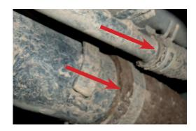
5. Remove check valve hose from tank.
