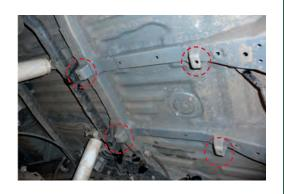
13. Unclip wiring loom form rear cross member to allow access to the body seam below loom.
