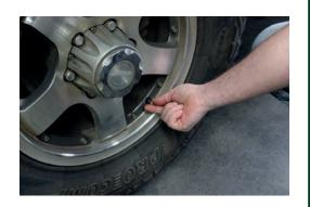
2. Attach Speedy Deflator to valve stem by supporting hose collar and rotating the valve stem adaptor in a clockwise direction.
