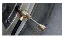
5. Push valve remover back in and screw in a clockwise direction until valve is tight.
