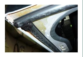
3. Inject silicone sealant into the hollow ends of rubber seals.
