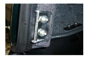
Catches also have slots and can be adjusted in and out by removing the plastic cover and loosening the retaining nuts.
