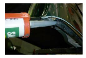
4 Apply a bead of silicone sealant between the ends of the canopy seals and the door seal.
