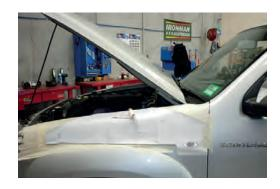
5. Using a felt tipped pen, mark all holes through template onto mudguard. Remove template.
