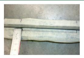
15. Remove section of trim by drilling a series of 3.5mm holes and cutting between holes to create a slot.
