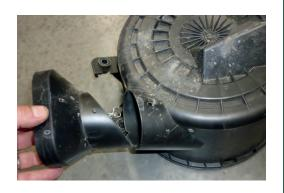
18. Position air cleaner adaptor over air cleaner intake and drill two mounting holes to 5mm.
