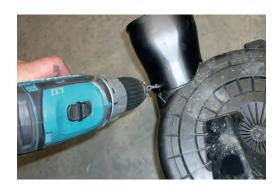
19. Seal adaptor to air cleaner intake using silicone sealant and secure in place using pop rivets provided.
