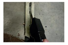
16. Refit plastic trim to pillar allowing bracket to pass through slot created in previous step (enlarge slot to clear bracket if required). Refit door rubber.
