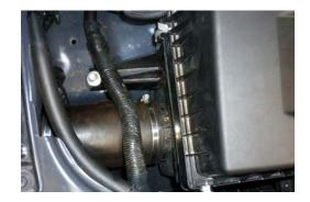
17. Apply a liberal amount of silicone sealant to inside of intake duct. Attach snorkel body to mudguard and secure with M8 Nylock Nuts and body washers making sure snorkel engages with air intake duct.
