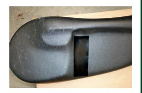
14. Place air intake duct in position under mudguard.
