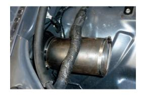
16. Refit air box and attach to rubber joiner.
