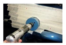
7. De-burr and rust-proof all holes (this applies to all holes drilled after this step).
