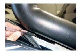
11. Drill mounting holes to 5mm. Remove mounting bracket from snorkel, apply silicone sealant to mounting holes and attach bracket to pillar using pop rivets provided.
