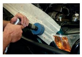
7. The bolt hole that secured the original overflow bottle to the inner guard in the engine bay will mark the centre of the 102mm hole required to be cut.
