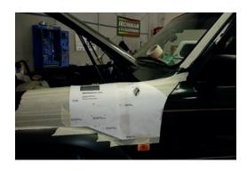
6. Using a felt tipped pen, mark all holes through template onto mud guard.
