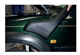
15. Slide connecting hose onto end of air entry duct with two hose clamps.
