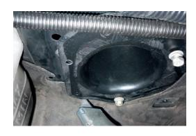
A. Drill three air cleaner mounting holes out to 11mm.
