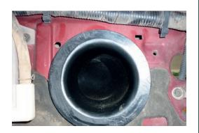
A. Remove foam seal from air cleaner inlet.
