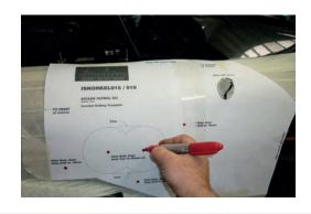
7. Using a 95mm hole saw, cut two semi circles as shown. Mark straight lines between the top and bottom of the semi circles and cut along using an air hack saw.
