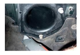
B. Remove plastic clip from mounting flange of factory air intake duct and drill hole out to 8mm.
