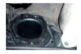
Secure duct to elbow using factory bolts and to air cleaner using hose clamp.
