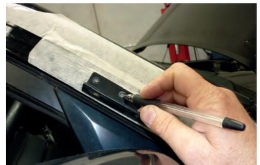
12. Install snorkel body to vehicle using M8 Nylock Nuts and body washers provided and attach to pillar bracket using M6 bolts provided.
