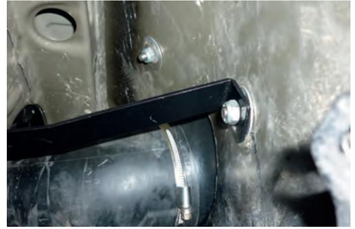
13. Attach rubber joiner to snorkel with outlet towards front of hole in engine bay and secure with hose clamp provided.
