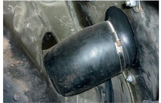
14. Remove foam seal from air box intake.
