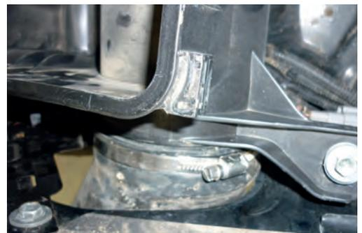
16. Check all hose connections and air box for potential leaks and seal as required.
