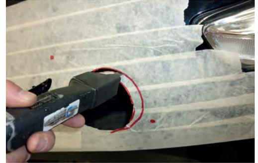
8. De-burr and rust-proof all holes (this applies to all holes drilled after this step).
