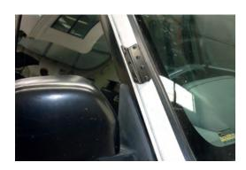
14. Install snorkel body top vehicle using M8 Nylock Nuts and body washers and secure to pillar bracket.
