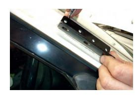
13. Apply silicone, insert mounting plugs and attach bracket using self tapping screw provided.
