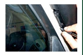
12. Remove pillar bracket from snorkel. Hold against pillar in position previously marked and mark mounting holes. Drill holes to 7.5mm.
