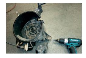
18. Apply a liberal amount of sealant to air entry hole in air cleaner. Refit air cleaner making sure air entry duct engages with air cleaner.
