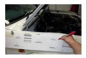
6. Using an 83mm holesaw cut two semi circles as shown. Mark straight lines between the top and bottom of the semi circles and cut along lines using an air hack saw.
