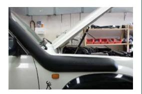
14. Attach rubber joiner to snorkel. Slide two hose clamps over hose but DO NOT tighten at this stage.
