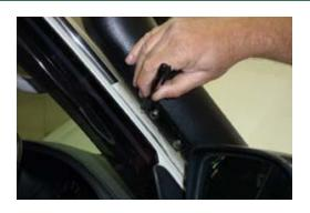
10. Remove bracket from snorkel, hold against pillar in position previously marked and mark three mounting holes.
