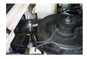
16. Secure rubber joiner with hose clamps.
