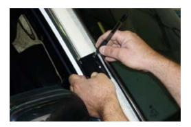
11. Drill three mounting holes in pillar to 7.5mm.
