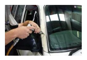
12. Attach pillar mounting bracket with three self tapping screws provided.
