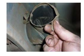
20a. Apply silicone sealant to inside or air entry duct to seal to air box elbow.
