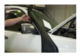
18. Attach rubber joiner to air entry duct and secure with hose clamp provided.
