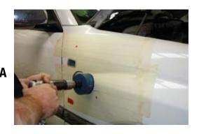
8b Using a air hack saw or similar cut a straight line between top and bottom of holes.
