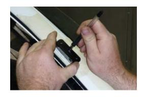
14. Apply silicone sealant to holes. Insert mounting plugs and attach mounting to pillar using self-tapping screws provided.
