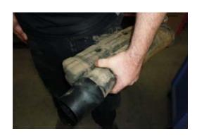
19. Remove foam seal from air box elbow under mudguard.
