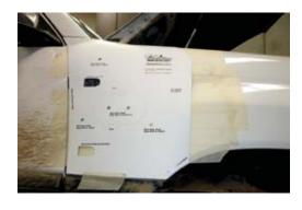
7. Using a felt tipped pen, mark all holes and new location for side indicator.
