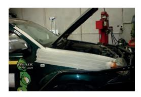
4 Tape template to mudguard making sure it is lined up with top of mudguard (bonnet opening) and rear of mudguard (door opening).
