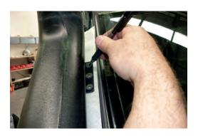
10. Drill mounting holes in pillar to 7.5mm. Apply silicone sealant. Insert mounting plugs and attach mounting bracket using three self tapping screws provided (When drilling mounting holes, only drill through outer skin and no further.)
