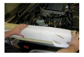
5. For vehicle without factory snorkel cut two semi circles holes using a 89mm hole saw as shown.
