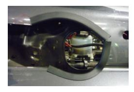
**10.** Using thread lock, screw all mounting studs into snorkel. Attach upper pillar mounting bracket as shown using M6 hardware.
