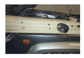
**8.** De-burr and rust-proof all holes (this applies to all holes drilled after this step).
