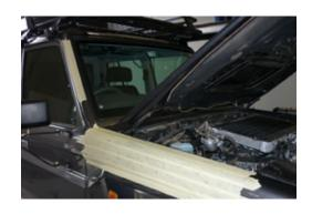
**4.** Hold template in position on the right hand mudguard and mark all holes and outer edges of two 'triangles' using a felt tipped pen or marker.
