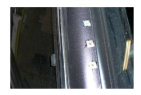
**13.** Attach snorkel to vehicle using M8 Nyloc nuts, body washers and self tapping screws for pillar bracket.
