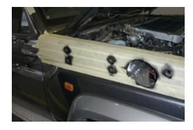
**9.** Apply rubber edging to large hole as shown.
