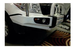
17. Once bull bar is aligned with vehicle and tightened, drill through pinning holes (circled in red) between bull bar and chassis bracket and secure with bolts, washers and nuts provided.
