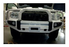
16. Align bull bar with vehicle and tighten all bolts.
