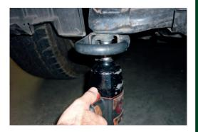
10. Attach mounting cradle to chassis as shown, reusing factory hardware.
