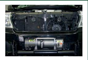
8. Bolt winch to cradle with gearbox to the left hand side of vehicle and cable spooling from bottom of the cable drum using bolts and washers provided.
