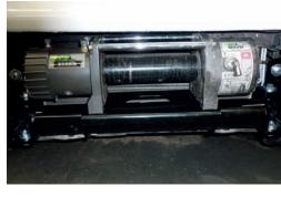
14. Connect the thin black earth wire and negative battery cable to the earth connection on the opposite side of winch motor.
