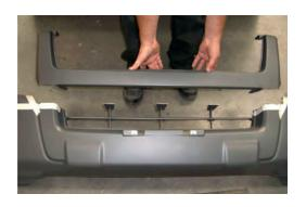
7. Fit chassis bracket to front of chassis using OE bolts and flat washers provided.
