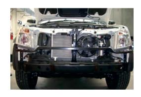
3. Remove inner bumper support brackets from radiator support panel.
