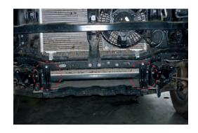
4 Trim outer bumper support brackets and mudguard liners level with bottom of radiator support panel.
