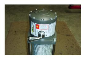
2. Undo and remove two chrome Allen head bolts which hold the gearbox to the tie rods.
