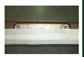
4b. Using an air hack saw or similar, remove lower section of bumper.
