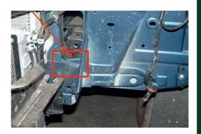
7. Secure chassis bracket to chassis using original bolts with heavy duty flat washers supplied to four upper mounting points and M12 x 1.5 x 40 flat washers and spring washers supplied into four mounting holes under chassis.
