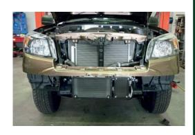
6. Place chassis bracket in position on chassis, making sure that bracket does not touch the vehicle body.
