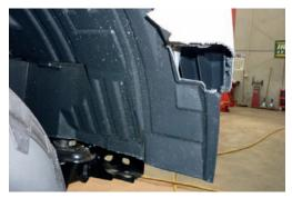
10. Remove steel bumper bar reinforcement.
