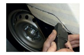
8. Install pinch weld to cuts on ends of bumper bar.
