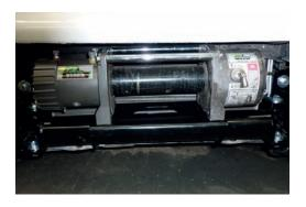
9. Bolt roller fairlead to recess in front of bull bar using bolts, washers and nuts provided.
