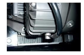
15. Run the positive and negative battery cables into the engine bay taking care to secure cables away from any sharp or moving objects.
