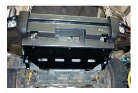
16. Trim mud guard liners level with protection plates and secure with cable tie.
