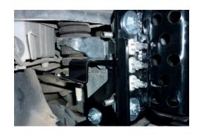
15. Fit protection plates underneath the bull bar using M8 bolts, spring washers and flat washers provided.
