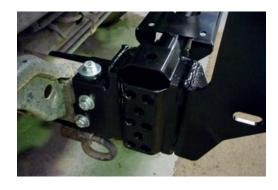
5. Refit recovery hooks using original bolts.
