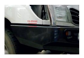
11. Once bar is aligned with vehicle and tightened, drill through pinning holes between bull bar and chassis brackets. Secure with hardware provided.
