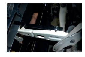
16. Fit protection plates underneath the bull bar using M8 bolts, spring washers and flat washers provided.
