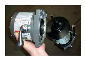
NOTE: If shaft comes out of cable drum remove it from the gearbox and place it back into the drum making sure it engages with the brake.
