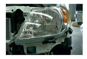
4 Remove plastic deflectors from between headlights and radiator opening.
