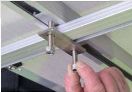
This diagram shows the rooftop tent clamped to a cross bar using clamp plate and bolts provided.
